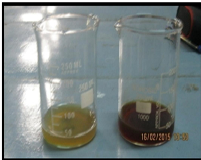
Figure No.1: B. Photograph showing both Flower extract and color change after adding \text{AgNO}_3 of P.tuberosa
